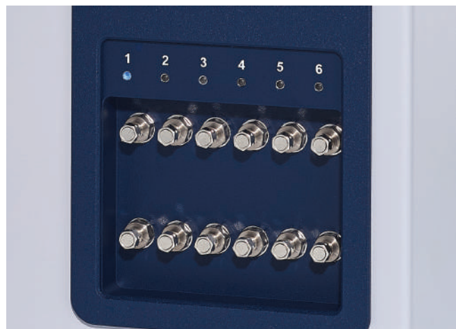
Internal 6-port multiplexer: the operating measurement channel is indicated with a blue LED
