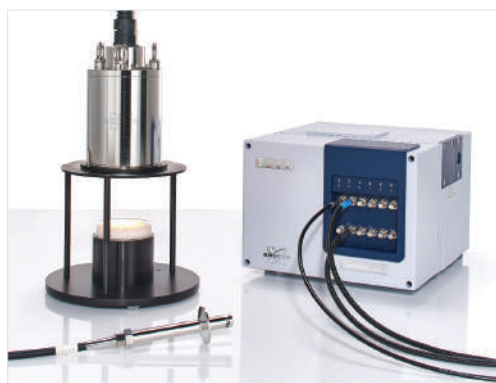
MATRIX-F II duplex: extension of the classical MATRIX-F II FT-NIR spectrometer for the simultaneous use of fiber optic probes and fiber-coupled sensor heads
