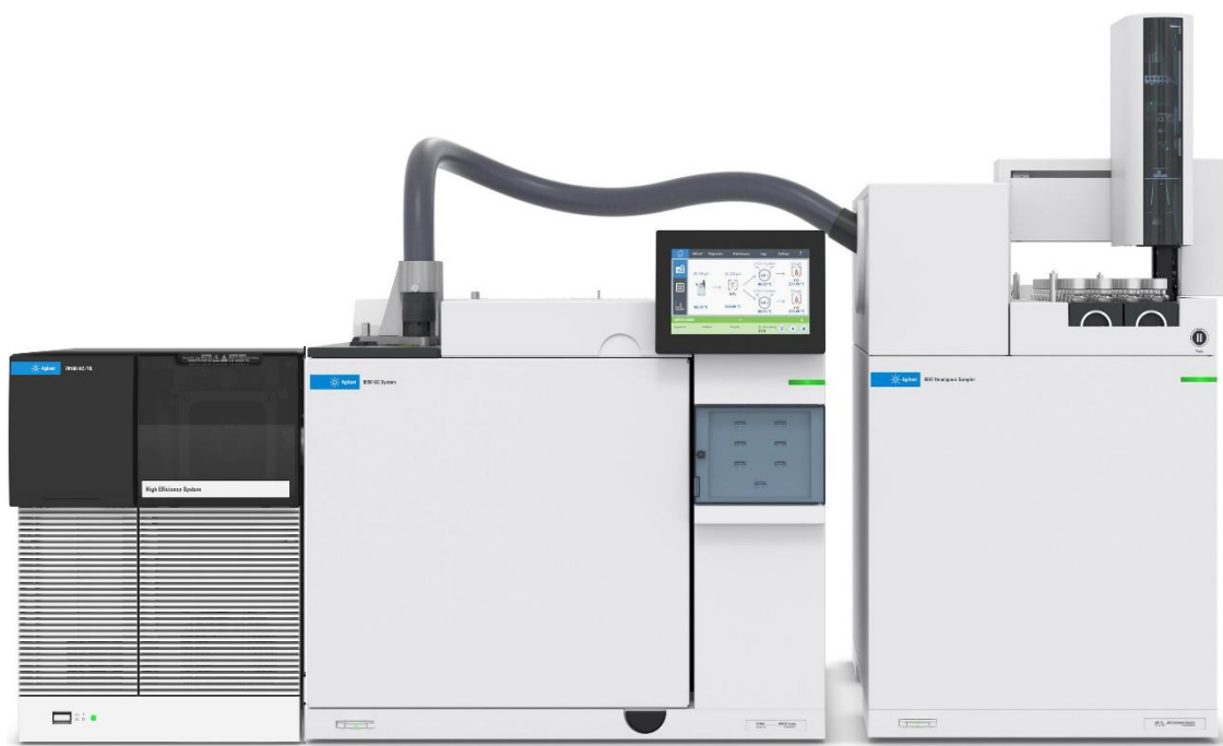
Figure 1. Agilent 8890 GC with 8697 headspace and 7010D TQ was used for this analysis.
